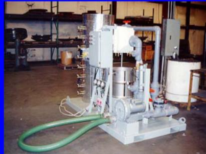
Mobile unit built by Tigg Engineering and tested at fumigation facilities on the East and West Coasts
