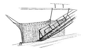
When the inboard end of a gangway or accommodation ladder rests on or is flush with the top of the bulwark, a bulwark ladder must be provided. Any gap between the bulwark ladder and the gangway or accommodation ladder must be fenced.
