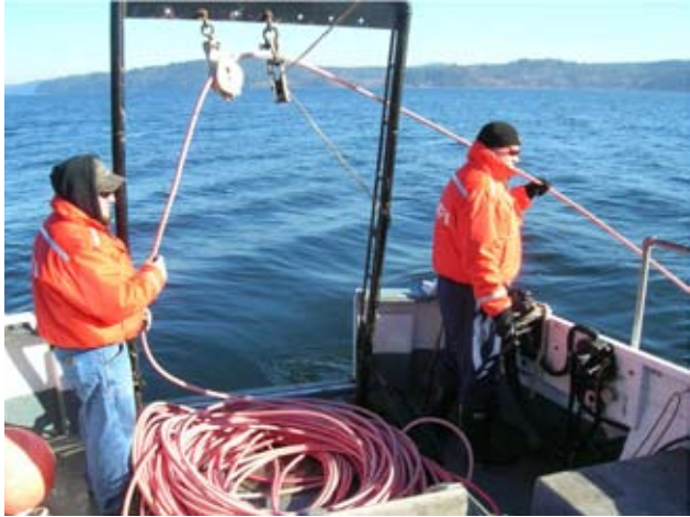
Figure 6. ROV umbilical coiled on deck of the R/V Molluscan .
