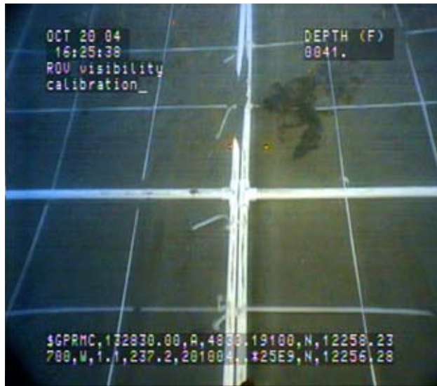
Figure 15. ROV calibration grid. Note laser dots for scale (10 cm separation).
