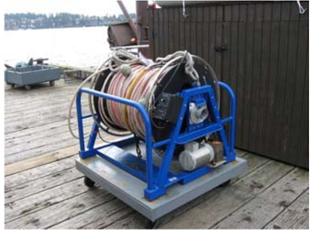
Figure 7. Motorized slip-ring and reel system for a Phantom umbilical. This unit is owned by the University of Washington Friday Harbor Laboratories.
