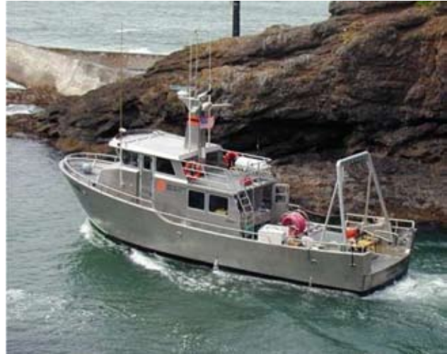
Figure 5. The R/V Elakha , owned and operated by Oregon State University. Note Phantom HD2+2 on rear deck and umbilical on reel behind cabin.
