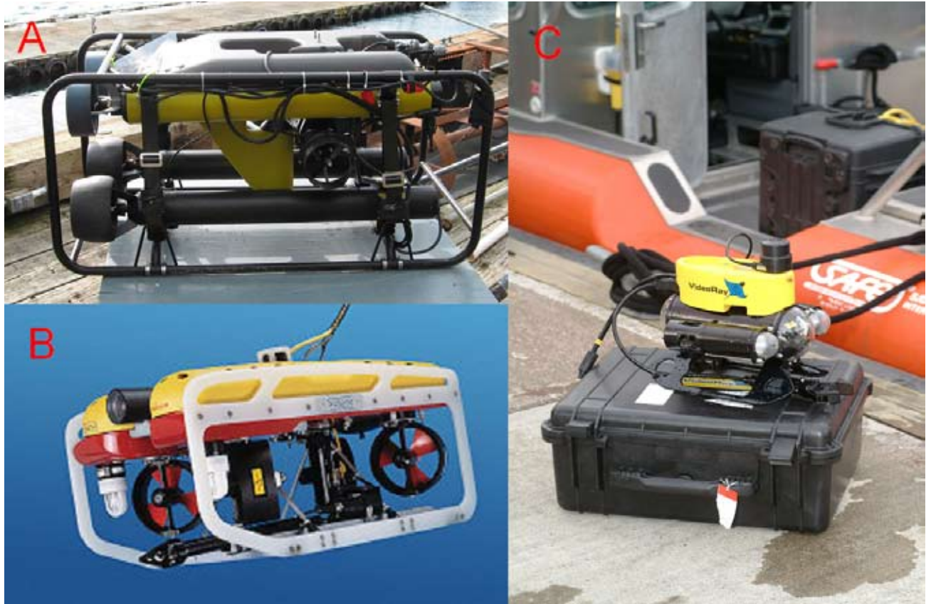
Figure 1. Examples of light-work and mini-class ROVs. A: Deep Ocean Engineering Phantom HD2+2. B: Seaeye Falcon. C: VideoRay Pro 3 XEGTO microROV.
