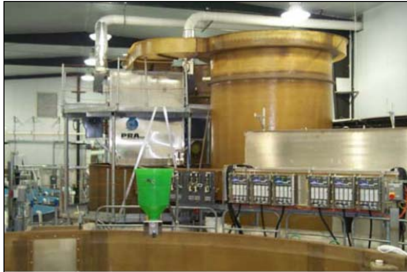
Figure 3. A RAS using a CycloBio Filter, Low Head Oxygenation (LHO) Unit and Stripping Columns. Water flow exiting the top of the fluidized-sand biofilter flows by gravity through a cascade stripping column, an LHO unit, and a UV irradiation unit before being piped by gravity to the culture tank. Photo courtesy of the Conservation Fund Freshwater Institute (Shepherdstown, WV).
