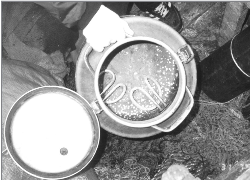
Home-made electrically heated pot used to boil illegally caught king crabs
