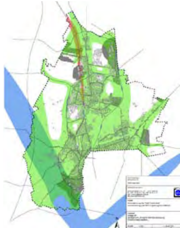
3 Lärmbelastungen in Norderstedt: blau = Fluglärm, grün = Straßenverkehrslärm, rot = Schienenverkehrslärm, grau = Gewerbelärm Noise exposure in Norderstedt: blue = air traffic noise, green = road traffic noise, red = rail traffic noise, grey = noise from industrial activity sites
