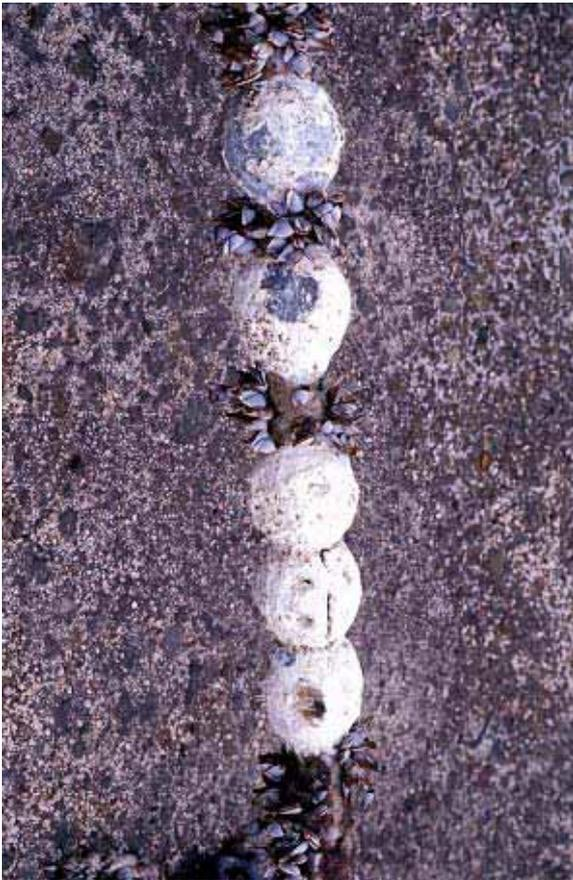
Anodes on the GRP MKII buoy, On the GRP buoy anodes will last for more than two years, even in areas with strong currents. On the stainless steel buoys anodes eat away much more rapidly and have to be replaced within a year. When the anodes are gone the shackles corrode very rapidly.
