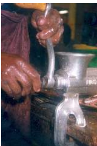
Photo 9: Mincer being dismantled for cleaning and washing.
