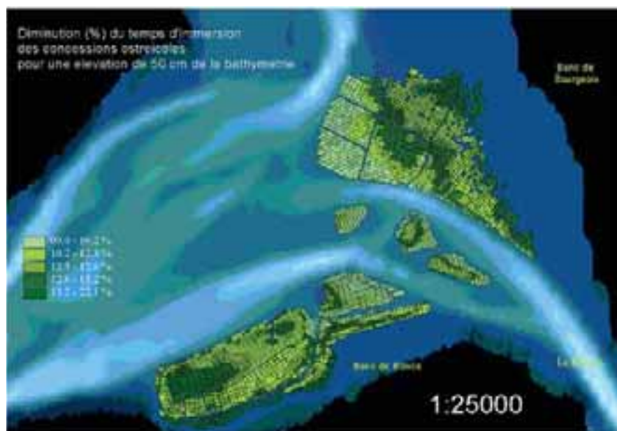
FIGURE 3.18 Loss of duration of immersion (in %) for a theoretical siltation rate of 50 centimetres on oyster lease grounds in Bancs de Ronce and Bourgeois
