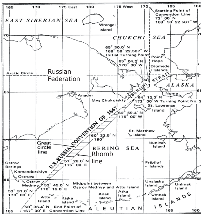
Figure 1 – Depiction of the Differences Between the Bering Sea Marine Boundary Using Rhomb and Geodetic Lines on a Mercator Projection
