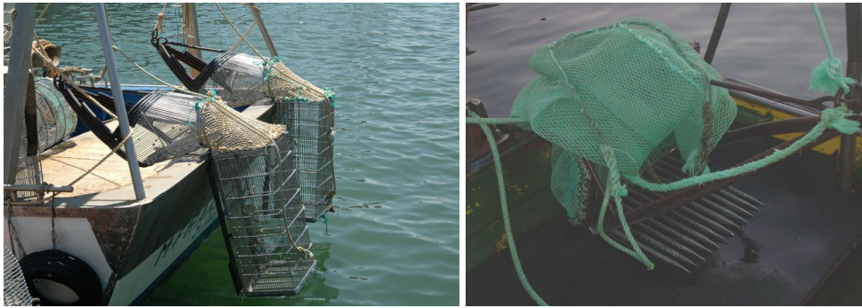
Figure 4.4-22 - Clam (left) and razor clam (right) dredges used in the Algarve bivalve fishery.
