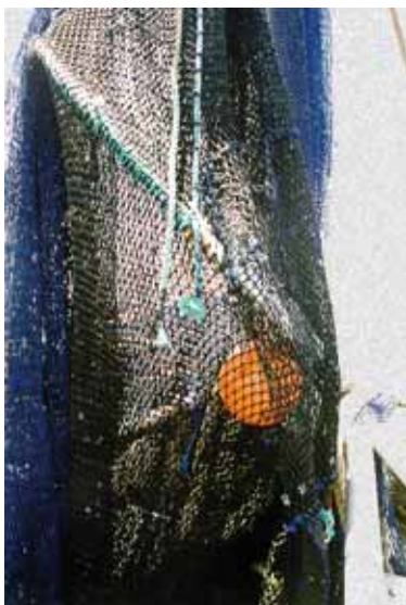
Belly ropes (lastridge ropes) are a simple option to prevent loss of grid angle, particularly as the meshes supporting the grid become worn and stretched.
