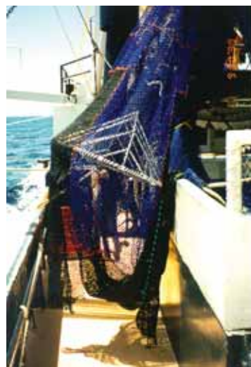
The pyramid TED was designed to exclude large animals through escape openings in the top and bottom of the codend. Shrimp loss was high probably because the grid is too small and the escape covers were attached too tightly to the codend.
