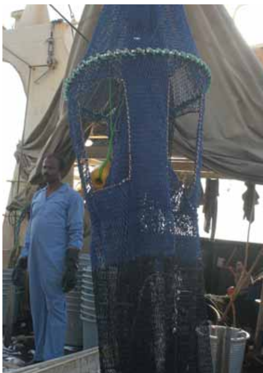
The design of the RES allows fish to swim forward in the codend and escape through the large escape openings.
