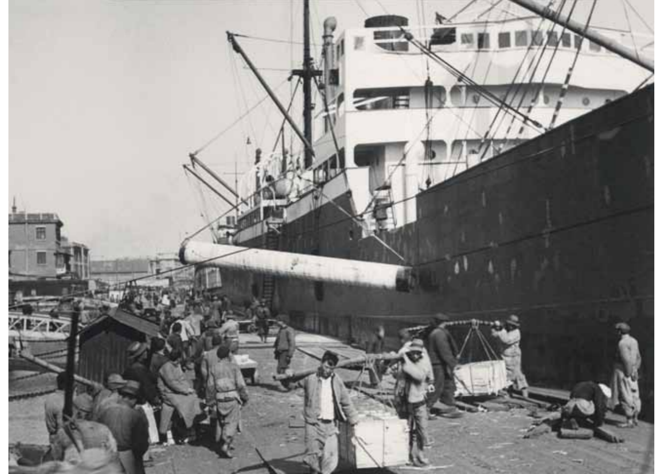
Cargo steamship BERTRAM RICKMERS in Asia in the 1930s. With no cranes on land, the freight had to be unloaded with the ship's own cargo lifting gear. Countless hands were required to carry the goods from the docks.
